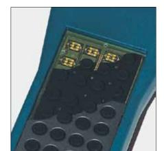
Switch mat set consisting of keypad plate, silicone switching mat and keypad circuit board with connecting cable
