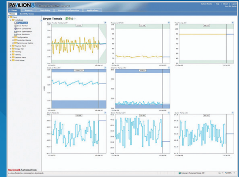
FactoryTalk Analytics Pavilion8 software's browser-based user interface provides easy access to monitor all aspects of the MPC solution.
