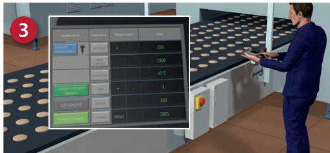
3. Operator informed about type of sensor and the location of it in real time
