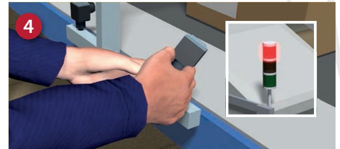
4. eBOM provides the device vendor data and part number for easy and fast replacement
