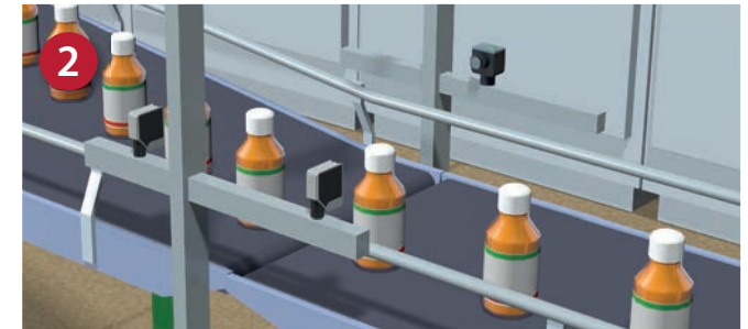
2. Smart Sensors configured on the conveyor with parameters for Product A
