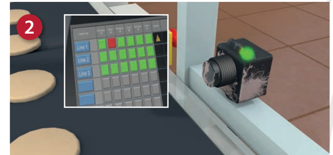
2. Sensor detects dust build-up
