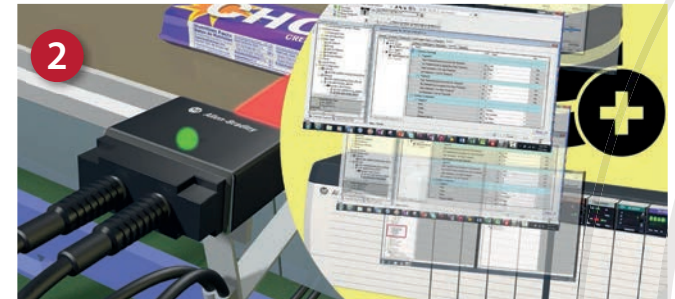
2. Connected to Logix Controllers over EtherNet/IP, and programmed by Studio 5000
