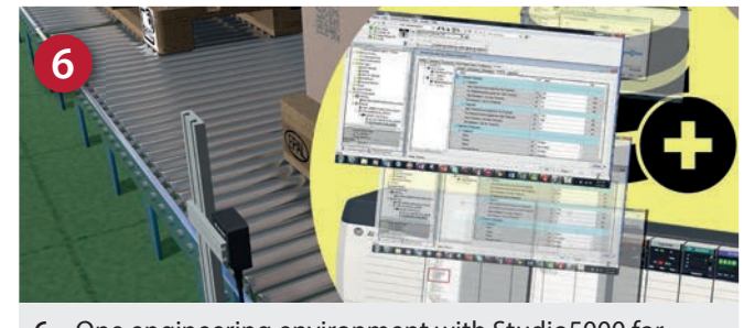
6. One engineering environment with Studio5000 for configuring and programming of all facets: Logix, HMI, Stratix 5700, PowerFlex, Kinetix, MES, Stratix 5700
