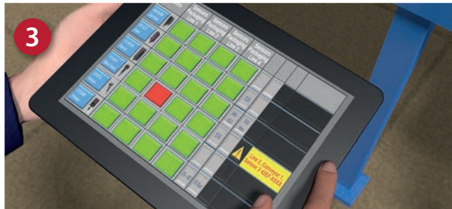
3. Application Specific Naming information (ASN) guides the operator directly to the fault
