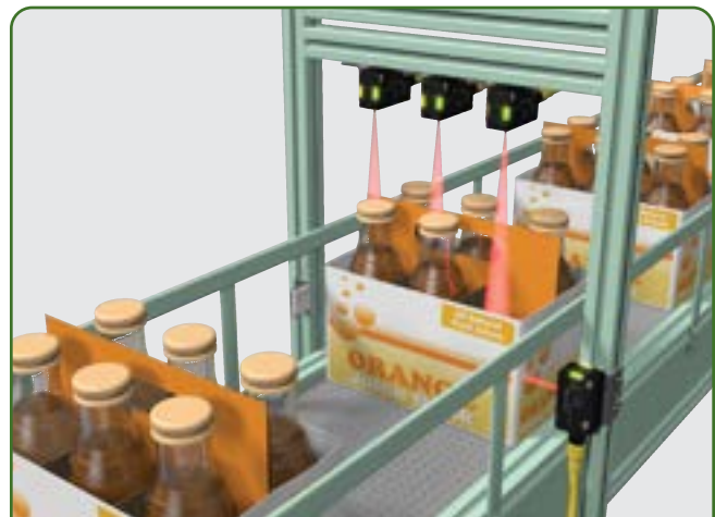
Bottling inspection - When the single 42JT LaserSight mounted on the side of the conveyor senses the bottle carton, it triggers the three standard VisiSights above to check for missing bottles.
