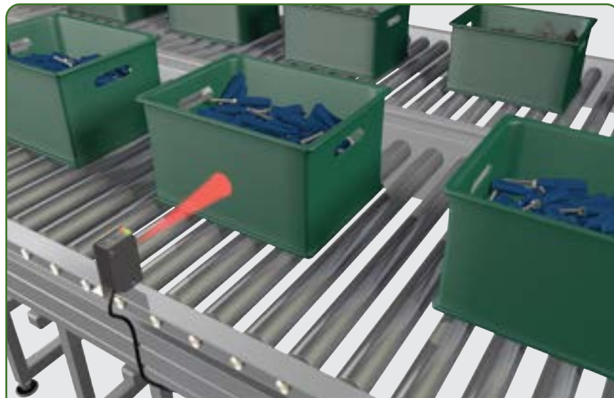
Side-by-side conveyors - A 42BT background suppression sensor detects bins on the near conveyor while ignoring bins on the second.
