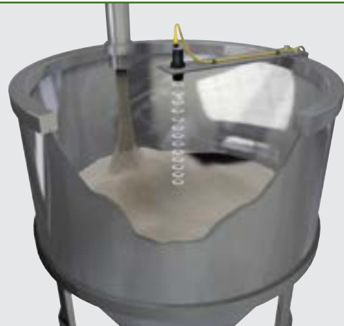
Roll diameter and tank level – An 873P analog ultrasonic continuously measures roll diameter or tank level and provides a proportional 4...20 mA or 0...10V DC output. If a dual discrete output sensor is used, one switch point is set for low level indication and the other set for a full condition.
