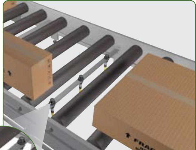
Material handling - Three 42CA sensors detecting boxes of varying sizes from below and in any position across the conveyor width.
