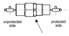
case / ground, torque max. 12 Nm
