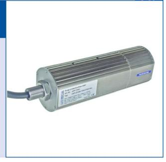
The Meteolabor USP-65001 surge protector / filter combines a multi-stage overvoltage protection for the two wires of a low voltage DC power supply with an integrated high quality filter for the attenuation of common and differential mode interferences.
