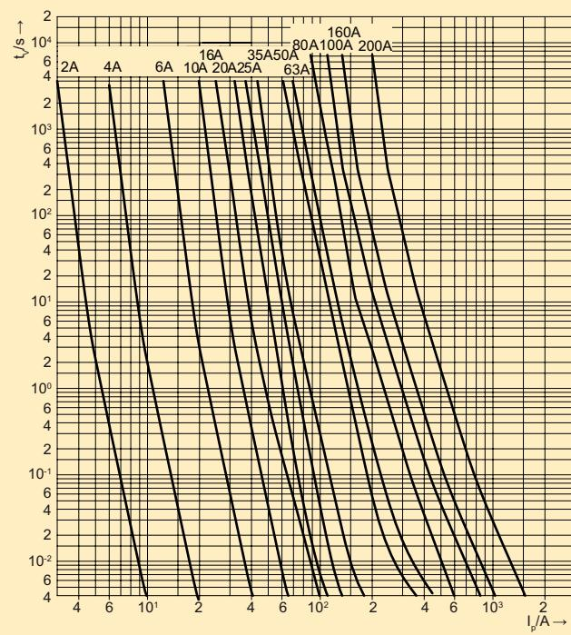
**Kennlinien gR AC400V-500V; D0/D / Characteristics gR AC400V-500V; D0/D****Strombegrenzungsdiagramm / Peak let-through current chart**
