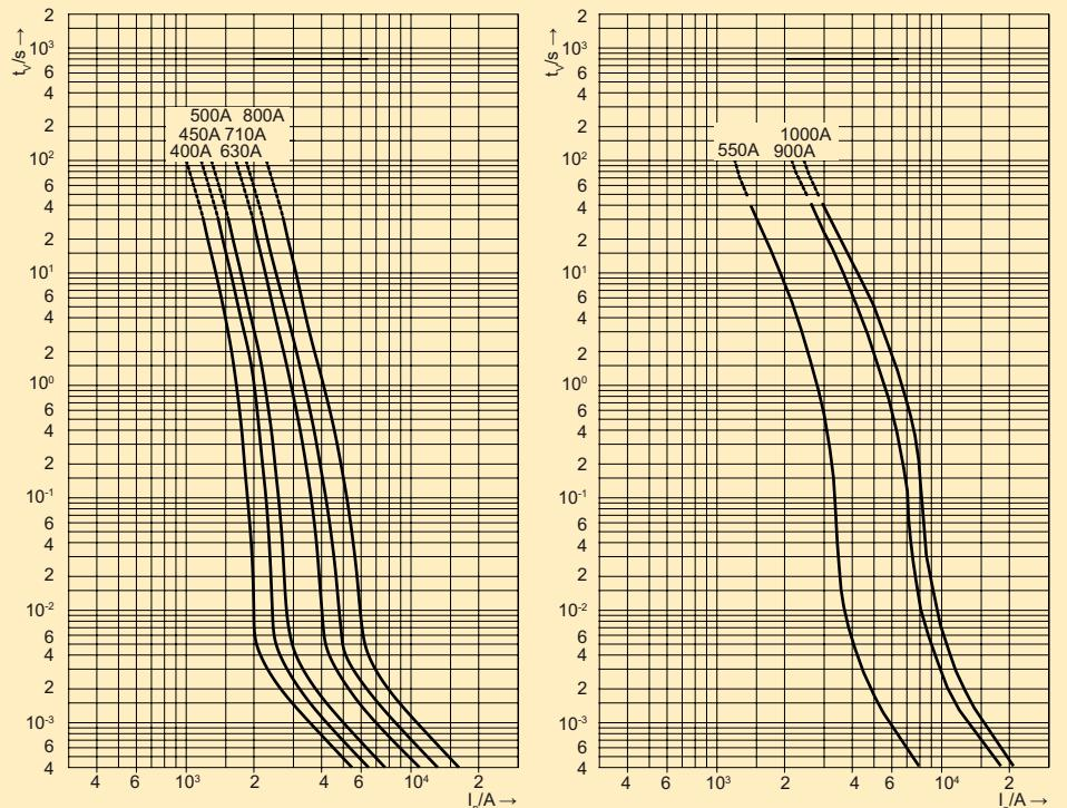
**Kennlinien aR AC690V / Characteristics aR AC690V****Mittlere Zeit/Strom-Kennlinie / Time current characteristics**
