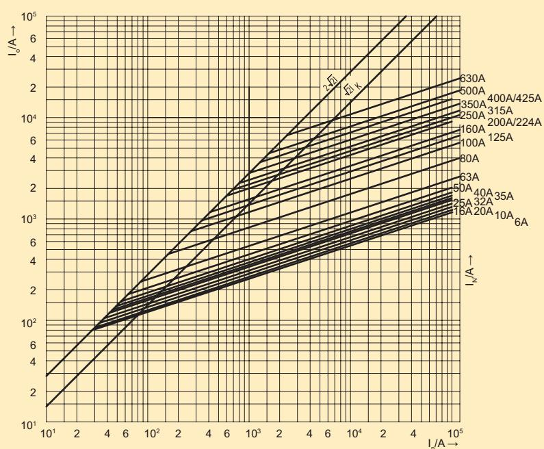
**Kennlinien gR AC500V-690V / Characteristics gR AC500V-690V****Strombegrenzungsdiagramm / Peak let-through current chart**
