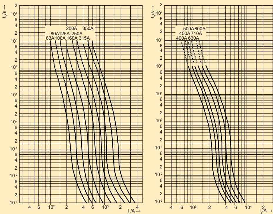
**Kennlinien aR AC690V / Characteristics aR AC690V****Mittlere Zeit/Strom-Kennlinie / Time current characteristics**
