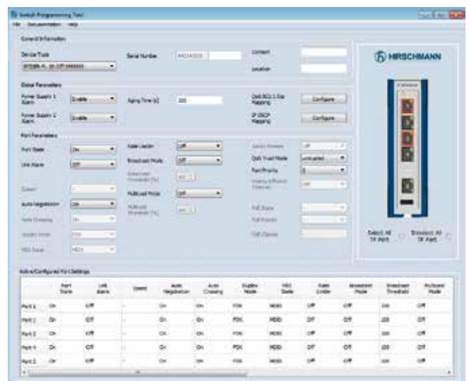
The stand-alone SPIDER Switch Programming Tool runs without installation (even from a USB drive), allowing for the customization of each individual port to the application's needs.
