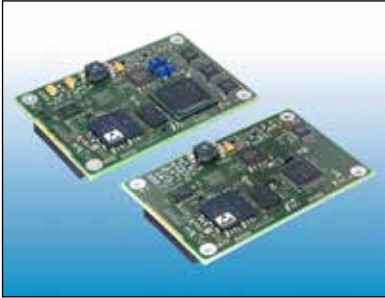
Example of Embedded Ethernet Switch EES25 on development kit
