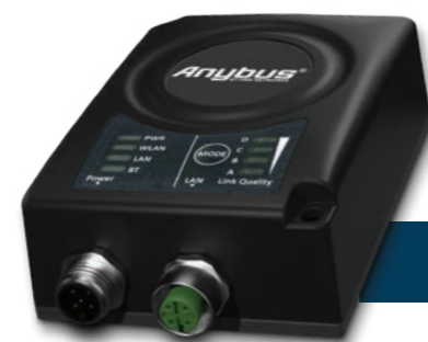
Ethernet over Bluetooth and WLAN Point-to-point or multipoint
