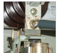
Testing with screwed-on V-shaped electrode
