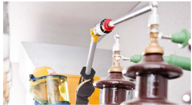
PHE III indicator with test prod, universal gear coupling and insulating stick
